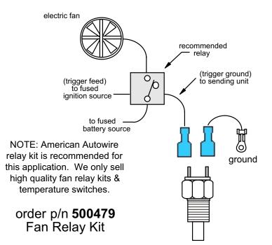
Apply anti-seize compound to the female threads in cylinder head or manifold before installing your new sensor. DO NOT overtighten! Sensor has tapered standard pipe thread (NPT) that self seals by design. DO NOT use pipe sealants or teflon tape. Use only with coolant containing corrosion inhibitors or antifreeze. Damage to sensor from overtightening or excessive corrosion voids warranty.
